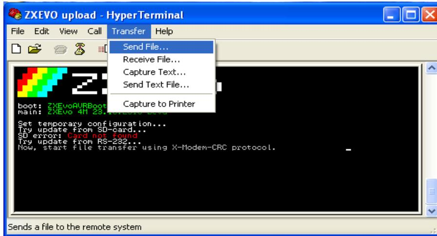
6. Select file with configuration (ZXEVO\_FW.BIN), set protocol «X-Modem» and press button “Send”.
